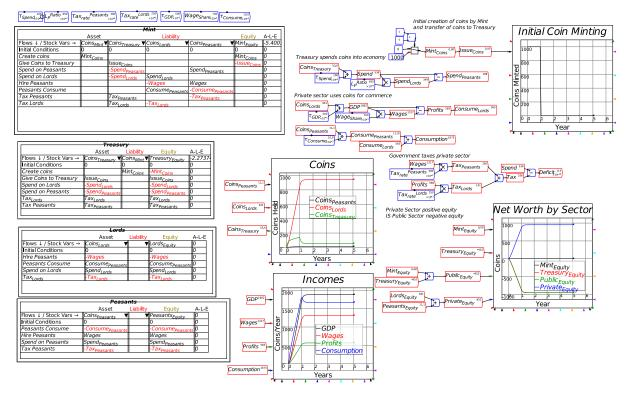
The Godleys Tab, with display of values turned on via the Options/Preferences menu, provides a nice overview of the flows in the model—see Figure 161. Notice that the Mint has zero equity, while the Treasury has negative equity of 952 coins—and this is precisely equal to the positive equity of the private sector, which is 11 for the Peasants and 941 for the Lords.
