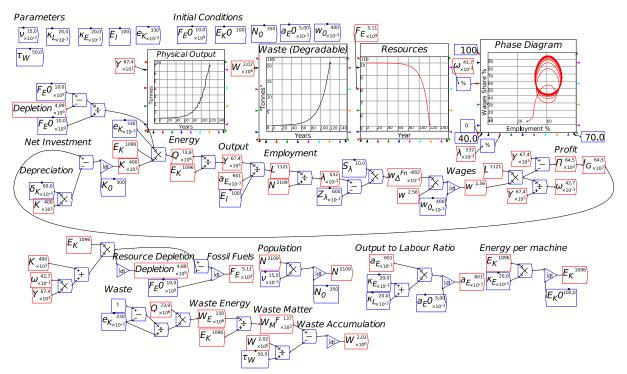
Figure 219: A Minsky system dynamics model of energy in production and resource depletion
