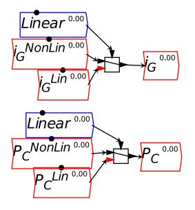
The switch function takes an input which can be zero or non-zero, and returns the first input if its value is zero, or the second if it is non-zero. The parameter *Linear* has an initial value of 0, a maximum of 1, and a step-size of 1, so it acts as the on-off switch. To make it easier to see what is happening, the indicator wire within the switch block will switch from one input to the other when the input condition is altered.
