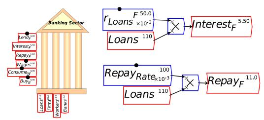
I prefer to use a time constant instead, because then the value of the time constant is easily understood in terms of the time dimension of the model. If I give that time constant a value of 10, as in Figure 116, then I get the same numerical result as in Figure 115, but the number 10 stands for the number of years it would take to reduce the debt to zero if this rate of repayment were sustained.
