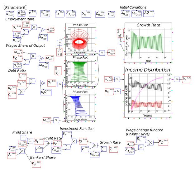
Figure 229: The Keen-Minsky model (same equations as (214) but with compact functions to save space)
