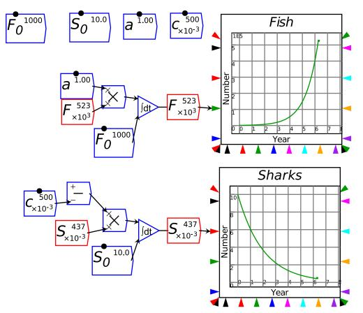
The model in Figure 83 also demonstrates one of *Minsky*'s shortcuts: to negate a number, simply feed it into the bottom port of a minus operator  $\begin{bmatrix} + \\ - \\ - \end{bmatrix}$ . With no input to the top port, Minsky interprets this as (0 - c) = -c.
