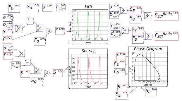
The final things needed to reproduce the figure in *Manifesto* is to replace the androgynous a, b, c, d parameters with more meaningful labels, and to put in the plot with the two Y-axes. We can do the former quickly using the right-mouse button menu item "Rename all instances"—see Figure 87.
